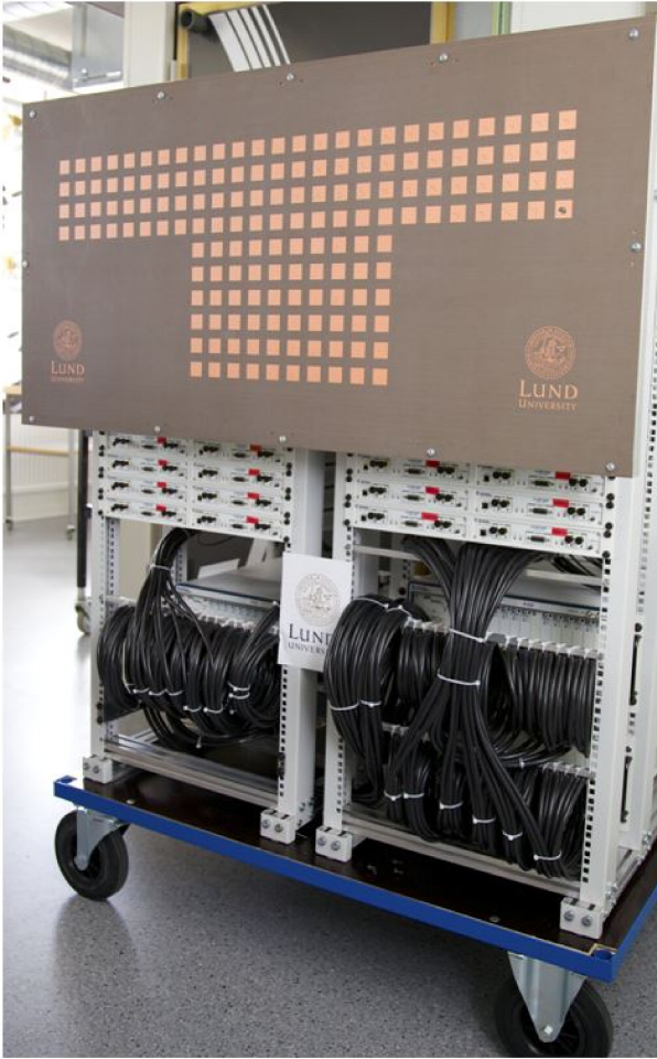
(a) Custom cross-polarised patch 100-antenna array developed in Lund University, in association with National Instruments (reproduced from [35]).
