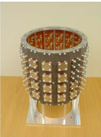
(c) 128-cylindrical array used to measure propagation characteristics for very-large MIMO at 2.6 GHz (reproduced from [41]).
