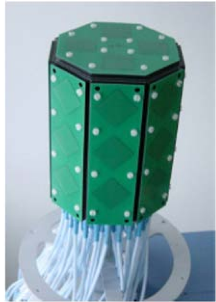
(b) 25-antenna array presented as part of METIS project optimised to function in the 2.3 GHz band (reproduced from [46]).
